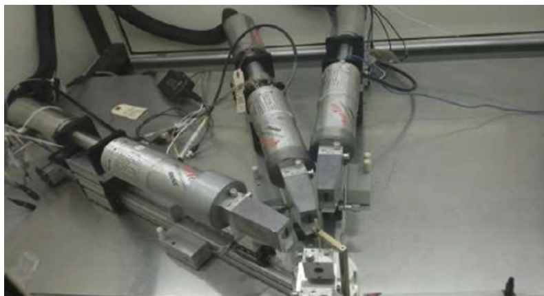
Fig. 2. The new EDXD diffractometer with three simultaneous detectors.
