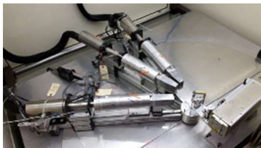
Fig. 2. EDXD_3H, the new EDXD diffractometer with three simultaneous detectors.
